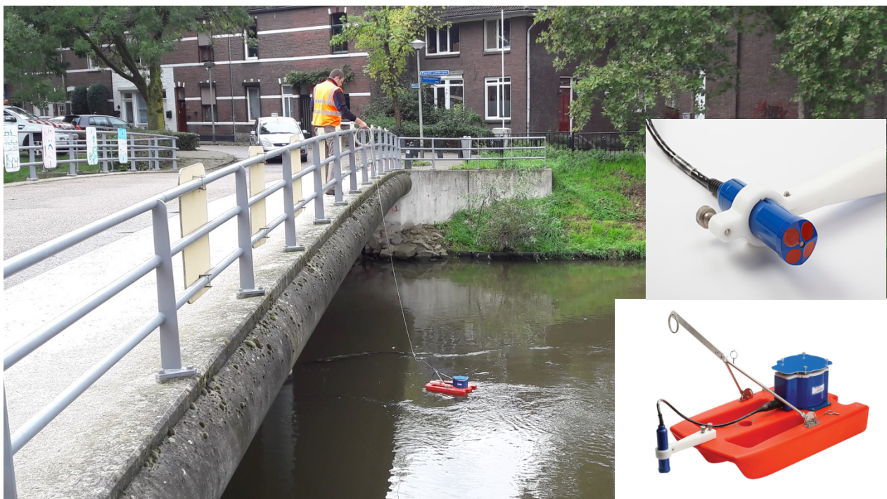
Figure 9 – Streampro ADCP operated on Voedingskanaal from bridge with details of instrument (Source: Google Maps – white paper - RD Instruments)
